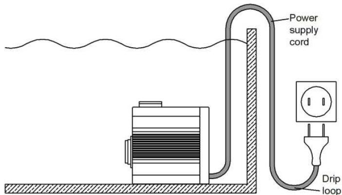
If the plug or socket does get wet, **DON'T** unplug the cord. Disconnect the fuse or circuit breaker that supplies power to the appliance. Then unplug and examine for presence of water in the receptacle.
